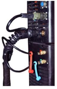
Installing water-cooled torch
