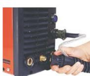
Installing gas-cooled torch
