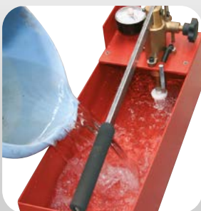
1-Fill up the tank
