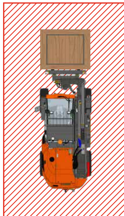
Dangerous areas around the machine.
