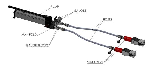
**Note:** A loose coupler will slow or stop the oil flow and is the most common cause of faulty operation.
