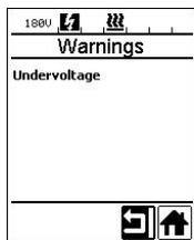
Warnings are displayed on a case-by-case basis in the **status display (31)**. If there is a warning pending, you can still continue to work largely without restrictions. The Warnings menu indicates the type of malfunction. Once the malfunction has been rectified, the entry disappears.
