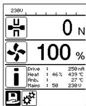
All available information (symbol *i*) is now displayed in the **working display (29)** (see Display symbols of the working display). The information field is always displayed below the field for the air volume.
