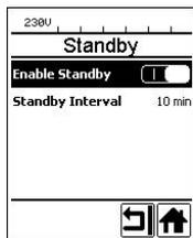
If the engine is switched off, the heating is activated, and if no key is activated during the time defined under Standby interval, then the device will switch over automatically to the Standby display. If the “e-Drive” (27) is not pressed during the subsequent 180 seconds, then the heating will automatically switch to Cool down mode. Standby will then appear on the display. Pressing “e-Drive” (27) causes the device to switch to Working mode.
