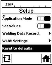
Use the **"e-Drive" (27)** to access the Setup menu and confirm your selection. Now set the Advanced Mode to On and then select Reset to defaults.
