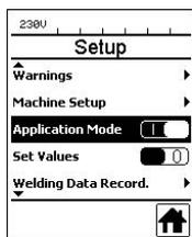
In the Basic setting, move through the Setup menu to save the profile, to Standby function, Application Mode, and Advanced Mode.
