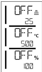
If the drive is switched off, then the welding parameters for temperature, air volume, and speed are set as follows in the **display fields (42)**:
