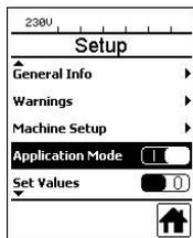
If you wish to have an overview of relevant information, e.g., line voltage, capacity utilization of the heating, select the Setup menu and confirm your selection. Now activate the Application Mode.
