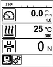
If you have activated the Set Values function, then the actual temperature (large) and the setpoint temperature (small) will be presented in the **working display (29)**. This will be in the analog form for the drive speed (m/min). If the function has been deactivated, only the setpoint values are displayed.
