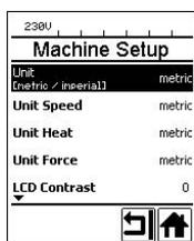
**Unit:** Setting the unit system (metric or imperial) for Unit Speed, Unit Heat, and Unit Force
